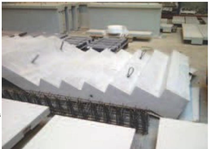
Ordered from specialist manufacturer of high-quality modular formwork systems and precast moulds, Cometal nv, the adjustable staircase moulds are used for casting straight run prefab stairs (Photo courtesy Portland Hollowcore).
