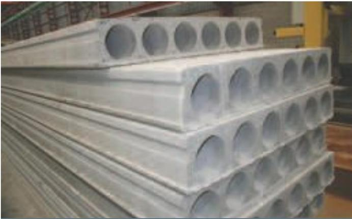
Hollowcore is cast with continuous voids to reduce weight and cost, and side benefit, for use to conceal electrical wiring or mechanical ducts.
